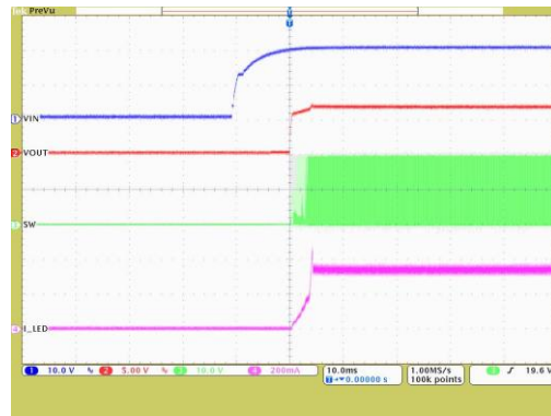
LED Dimming (50KHz) (VIN=24V, 1W-LED*2, I LED =350mA)
