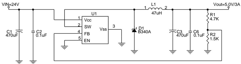
$$V_{OUT} = V_{FB} \times \left(1 + \frac{R1}{R2}\right), V_{FB} = 1.23V, R2 = 0.7K \sim 3K$$
