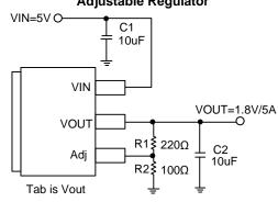
$$V_{OUT} = V_{REF} * (1 + \frac{R_2}{R_1})$$
