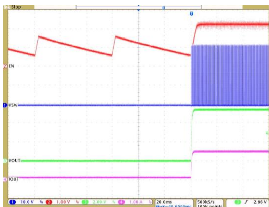
V CC =32V, V OUT =1.2V, I OUT =1.5A Thermal Shutdown Release
