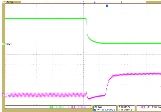
Short Circuit V_{IN}=12V, V_{OUT}=5V
