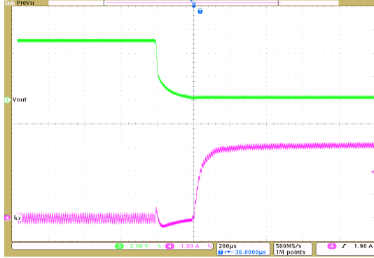
Short Circuit V_{IN}=12V, V_{OUT}=5V
